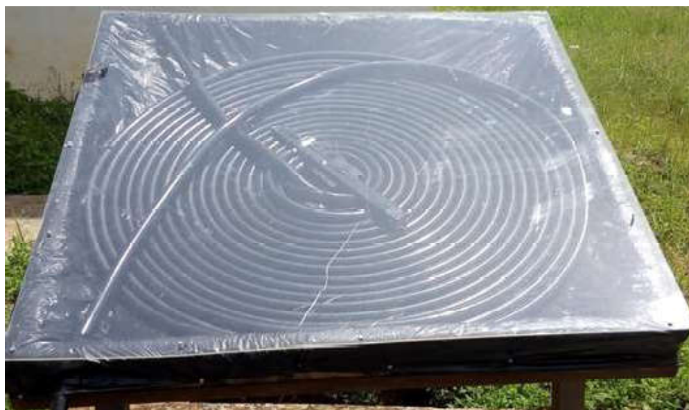
Figure 2: The solar collector system: The coiled hose of about 20 turn in a shallow box covered with a transparent glass.
